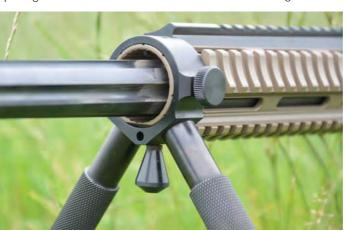
Having the bipod rotational axis in line with the bore aids stability before each shot and post shot aimpoint re-acquisition
