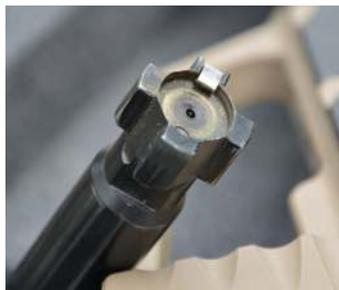
**Four lug bolt head with extractor and manual ejector. This responds directly to operation speed of the bolt, so faster cycling flings brass further**
