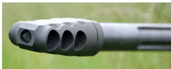
**A six-port Muzzle Brake is included, threaded on and clamped to remain indexed. Its directed blast area keeps noise well clear of the rifle's shooter**
