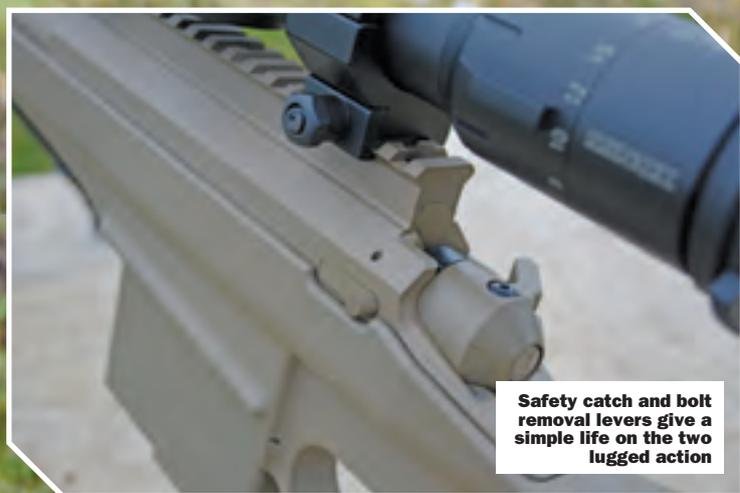
Safety catch and bolt removal levers give a simple life on the two lugged action
