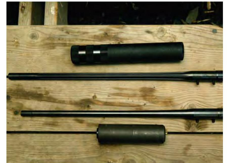
▲ There is a clear difference in length between the match barrel and moderator (top) and the standard hunting barrel and moderator (bottom). Weight and portability are also affected
