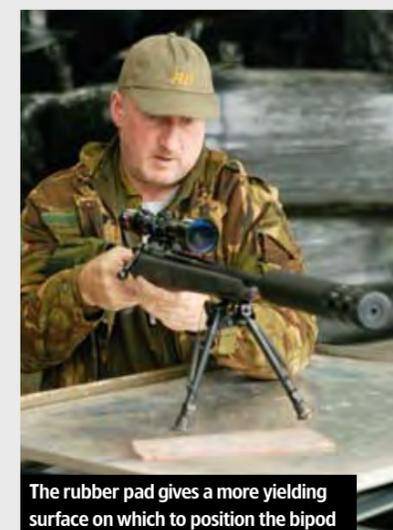
The rubber pad gives a more yielding surface on which to position the bipod
